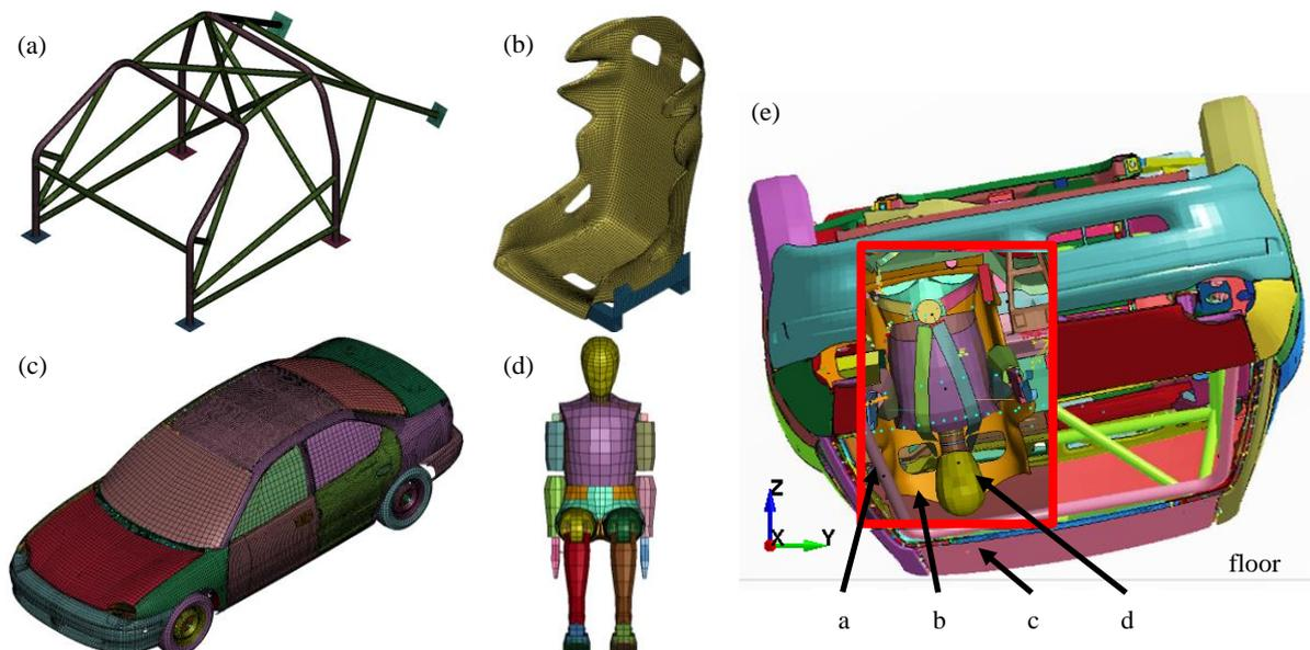
Figure 3. Meshed model of roll cage (a), seat (b) 1996 Dodge Neon and Hybrid III FAST (c) and 50<sup>th</sup> percentile male dummy (d) building simulation setup (e) showing harness
