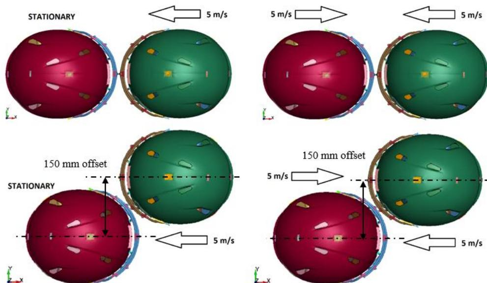
Figure 2. Impact configurations
