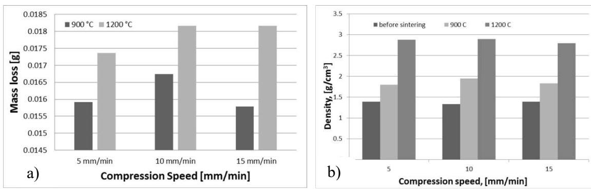
**Fig. 4. (a) Mass loss of hydroxyapatite disks after heat treatment;
