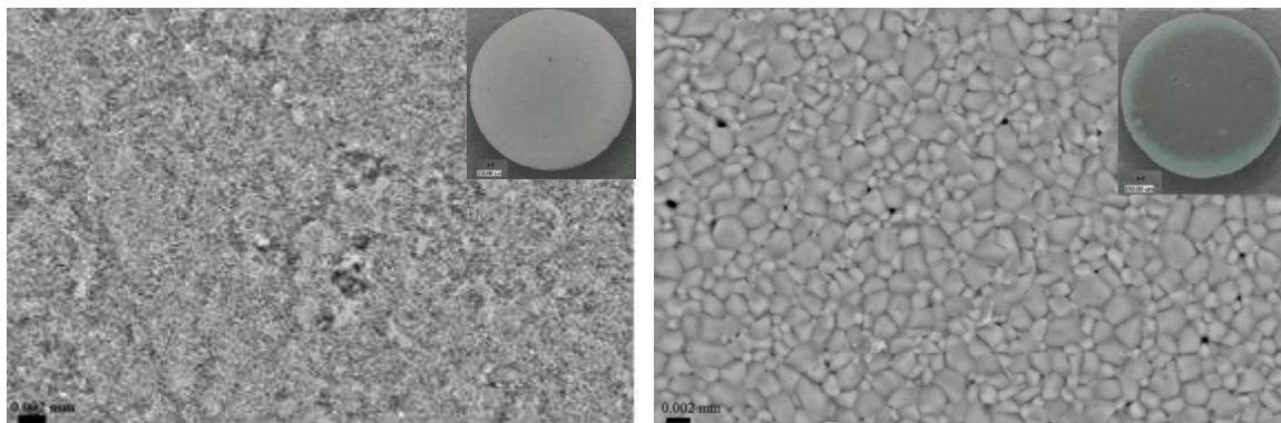
**Fig. 3. Structure of the pellet's surface, SEM. Left –  $900^{\circ}\text{C}$ , 10 mm/min; right -  $1200^{\circ}\text{C}$ , 10 mm/min**
