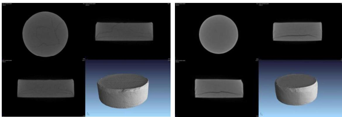
**Fig. 2. The results of non-destruction inner structure analyze by computer microtomography ( $\mu$ CT): left - pellet sintered at  $900^{\circ}\text{C}$ , 10 mm/min; right -  $1200^{\circ}\text{C}$ , 10 mm/min**
