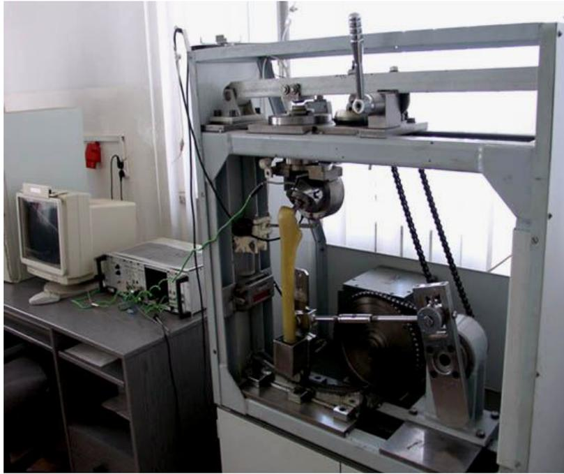
Fig. 2 Simulator to examine friction and wear of artificial joints
