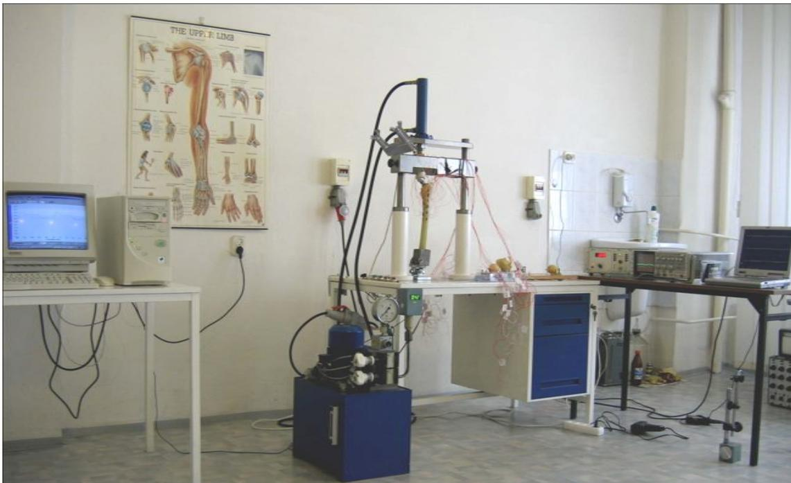
Fig 1. Femur bone placed on human hip joint simulator and connected to the measuring and recording device.
